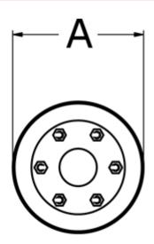
A = 82 D1 = 25 D2 = 25 L = 78 Nom. torque NM (Tkn) = 80
